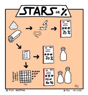
When we certify raw material, components or constituents, we perform several measurements to improve the accuracy of the biobased carbon content and TC/TOC, as these will be used to determine the biobased content of the finished products.
